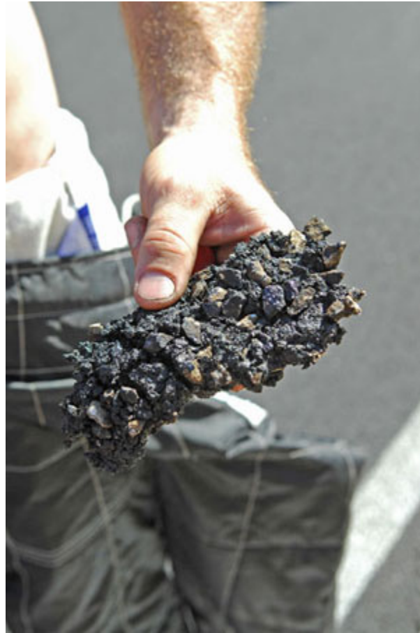
Above: Tyson Pearce shows a piece of race track. With chunks of debris like this coming off the surface, officials had no other option than to abandon racing. pic - Ash Budd, photowagon.com.au
